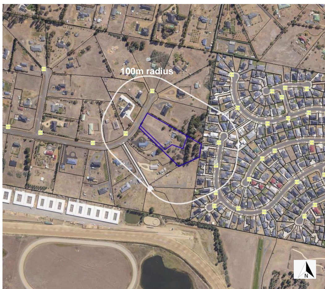
Figure 1: contoured listmap. www.thelist.tas.gov.au Subject property and proposed lot structure outlined in blue. Yellow squares represent mains fire hydrants.
