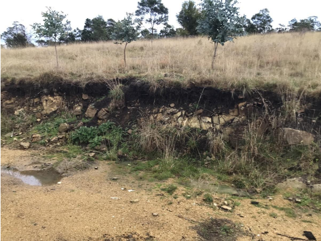
Figure 6 Belmont soil association black dermosol clay loam soil present throughout much of the property
