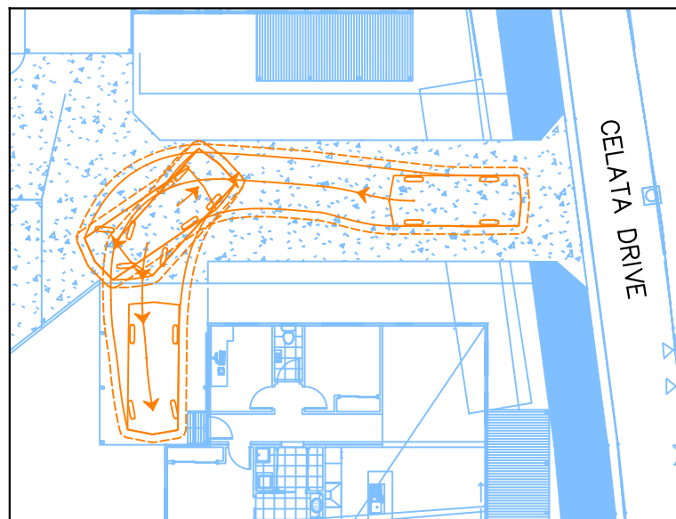
DWELLING 17A CARPORT ACCESS - 1
