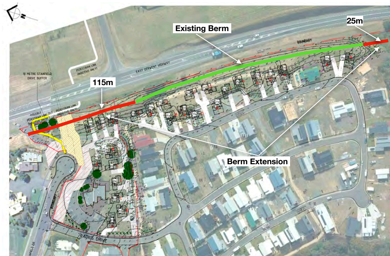
FIGURE 4.1: EXISTING AND PROPOSED BERM LOCATION
