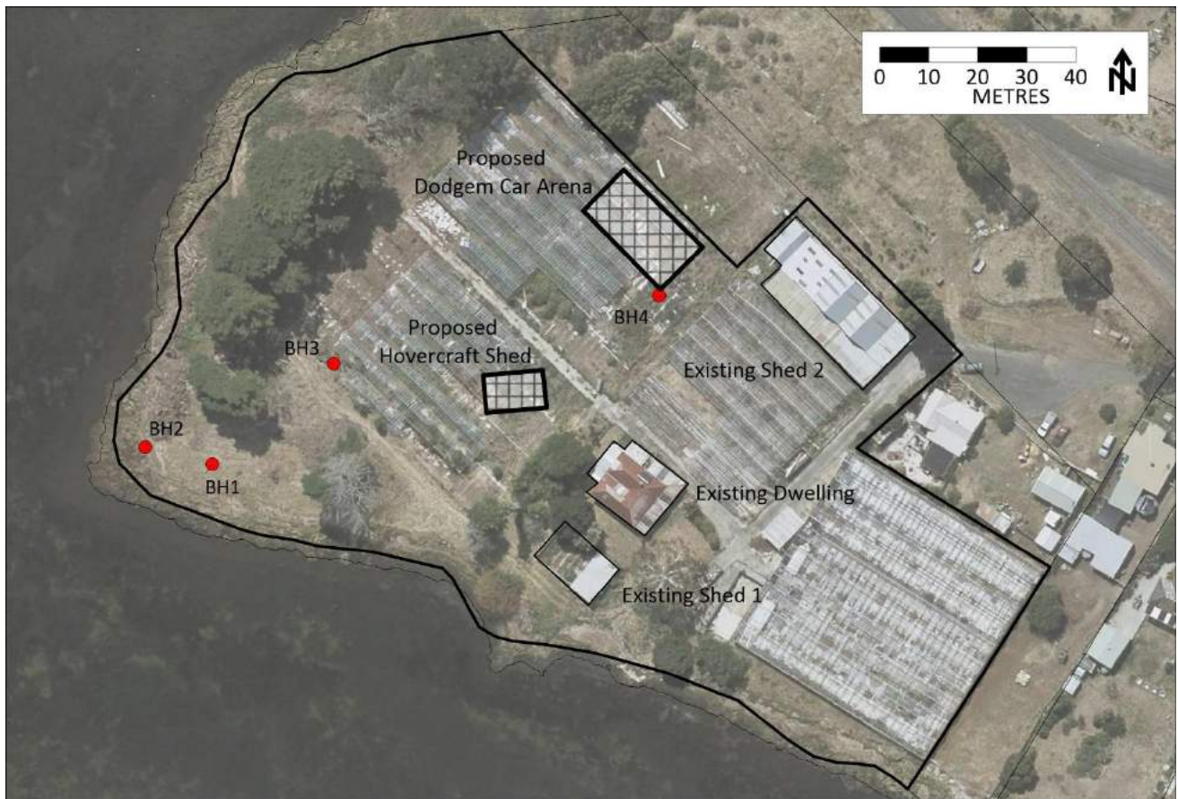
Figure 6 Site Layout & Borehole Locations
