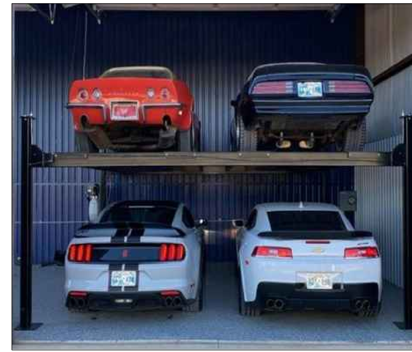
FIGURE 3 TWO STOREY VEHICLE STACKER
