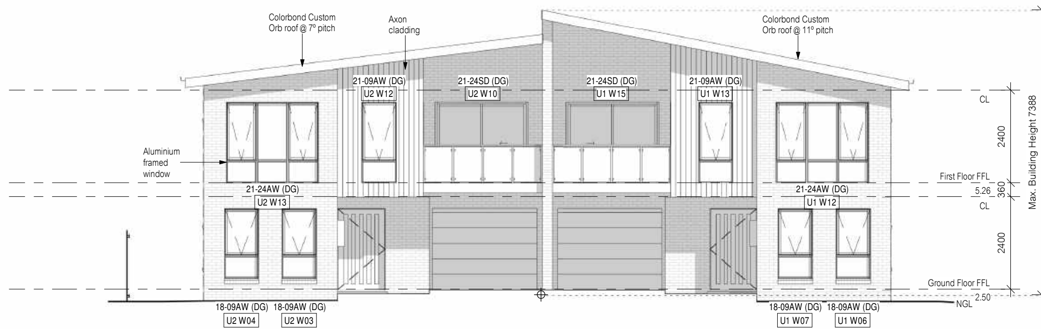
UNITS 1 & 2 SOUTH ELEVATION
