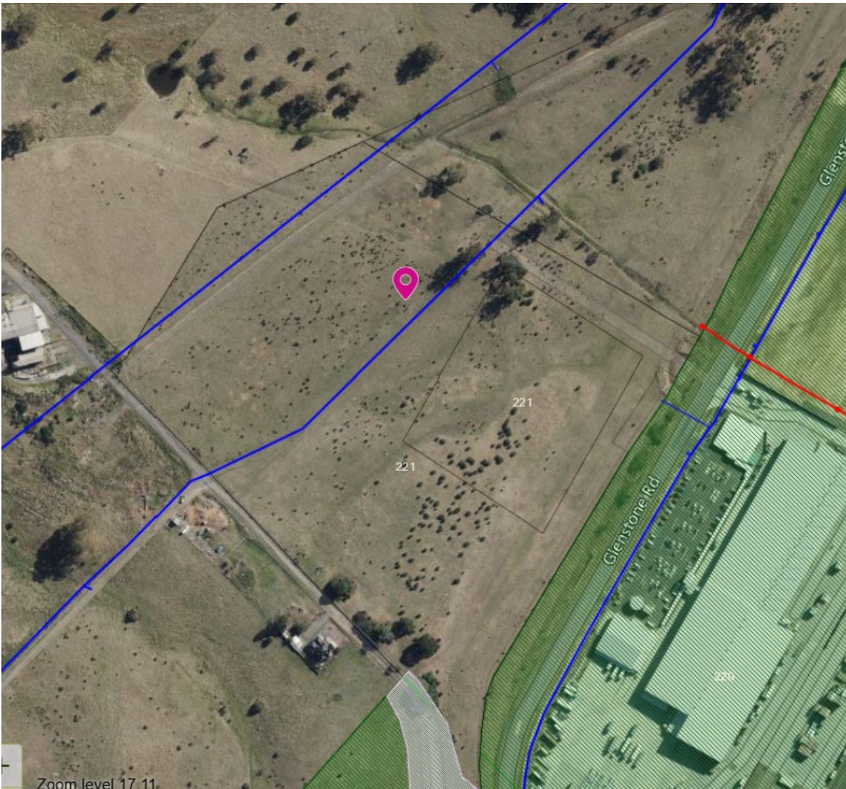
Figure 8: Access to Infrastructure servicing (reticulated water – blue line; reticulated sewer – red line)
