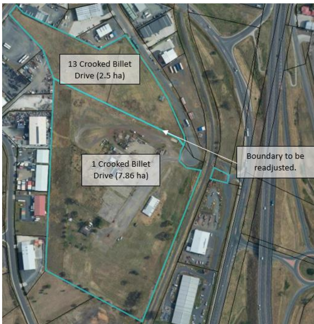
Figure 1: The boundary to be readjusted, delineating 1 Crooked Billet Drive from 13 Crooked Billet Drive ( List Map 2023 ).
