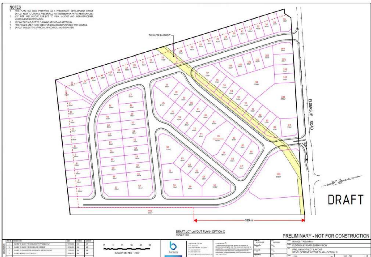
Figure 1 - Subdivision Civil Works Plan
