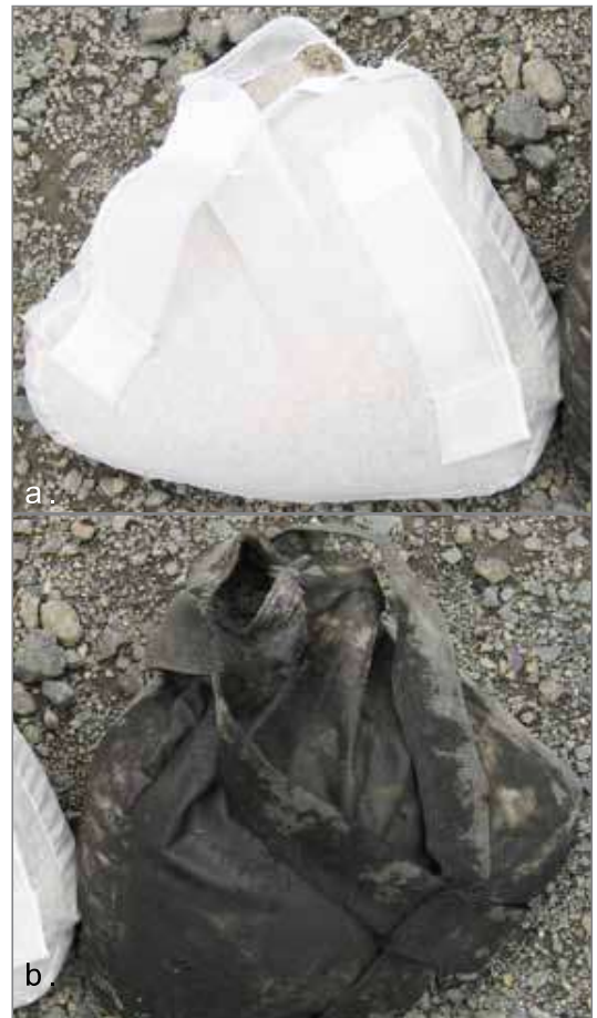
Fig.4 a) A new Media Bag of Hydro Filter Sand. b) A spent media bag of Hydro Filter Sand.
