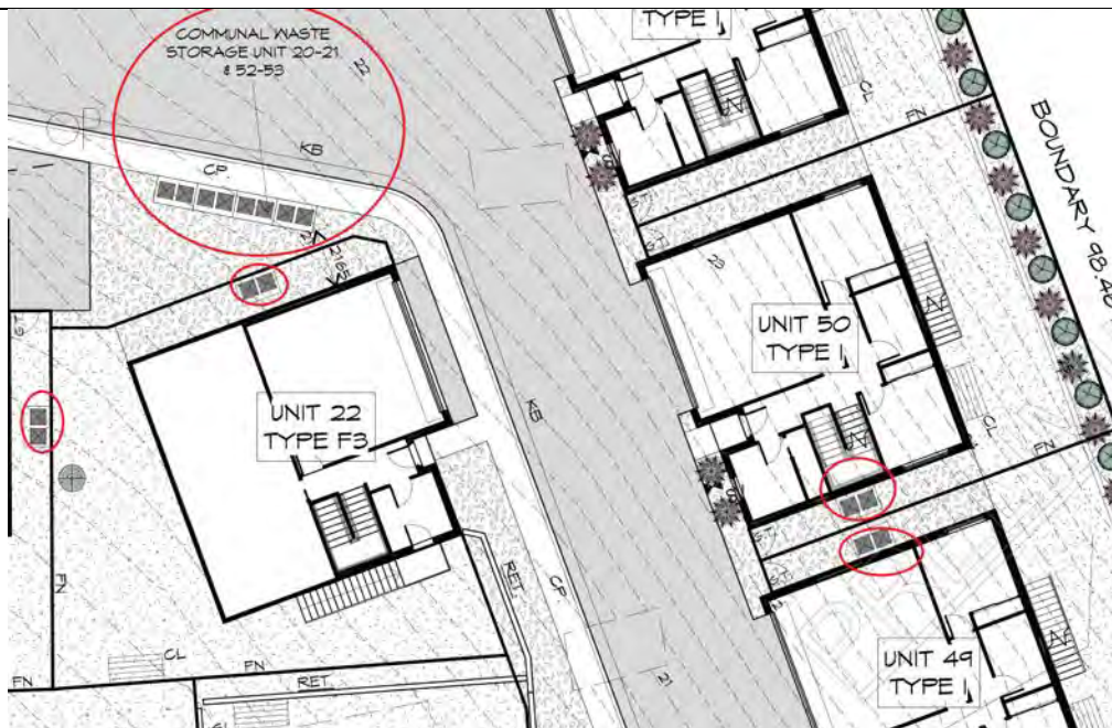
Example of the proposal for each dwelling to either have a designated bin storage area for exclusive use by that dwelling or access to a designated communal bin storage area.
