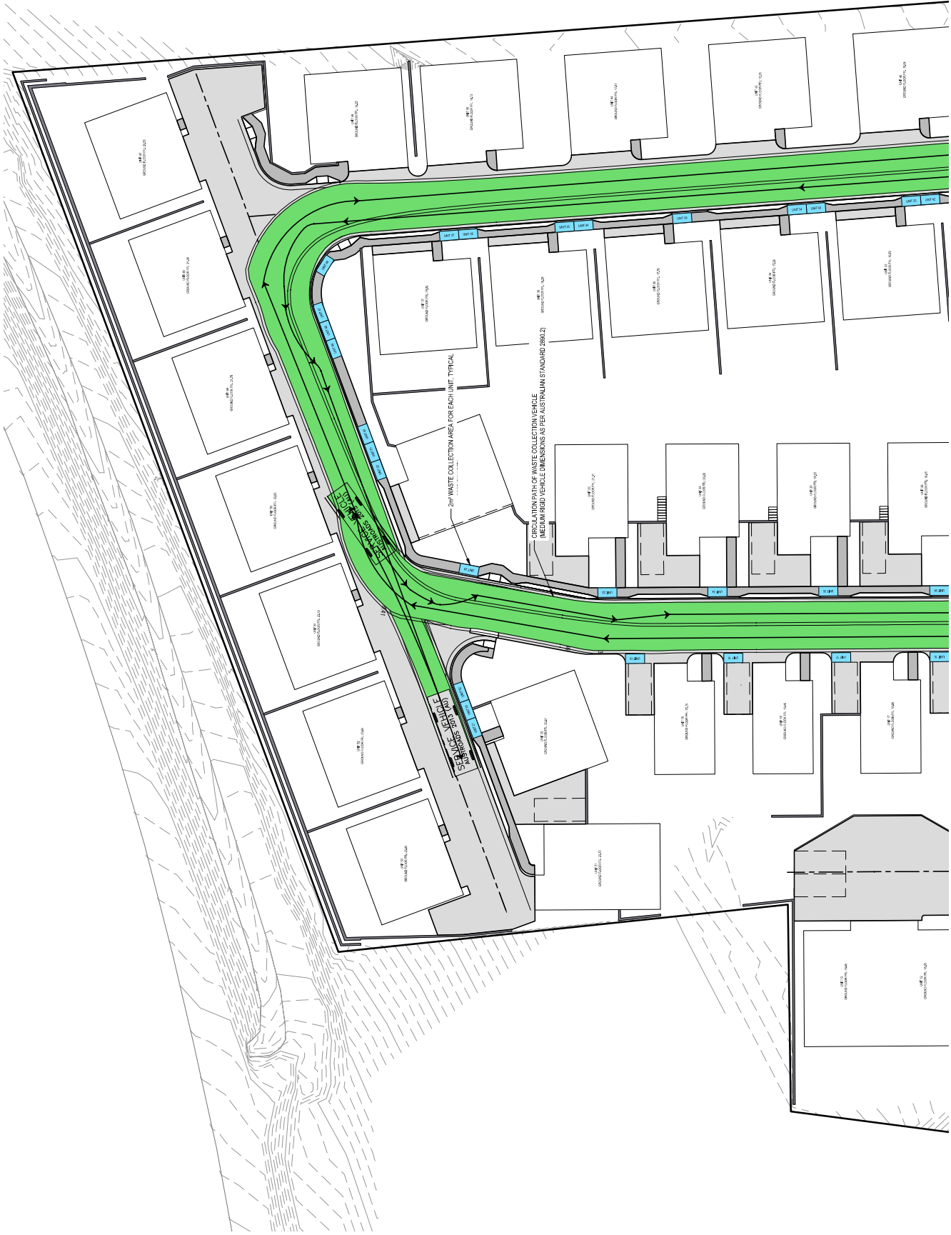
MEDIUM RIGID VEHICLE TURNING PLAN - SHEET 2 SCALE 1:200
